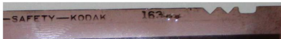
Acetate Kodak notch code (at right) and printing
