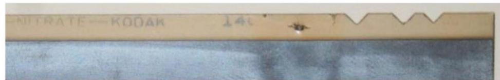
Nitrate Kodak notch code (at right) and printing
